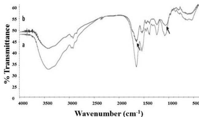
**Fig. 5.** FT-IR spectra of lyophilized biomass of strain Q5-1. Strain Q5-1 was incubated for 48 h (a) without Cr(VI) and (b) with the addition of  $125 \text{ mg L}^{-1} \text{ Cr(VI)}$ . The arrows show shifted peak.
