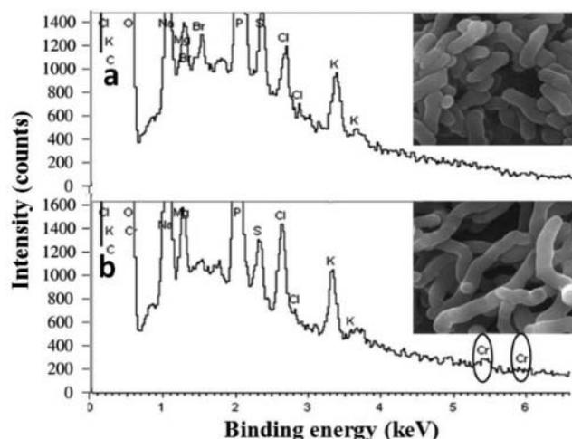
**Fig. 3.** EDS analyses for strain Q5-1 interacted with Cr(VI). EDS spectra of strain Q5-1 incubated for 48 h (a) without Cr(VI) and (b) with the addition of 125 mg L<sup>-1</sup> Cr(VI). Oval circles indicated the presence of Cr. Insets of (a) and (b): SEM images of strain Q5-1 used for EDS analysis.
