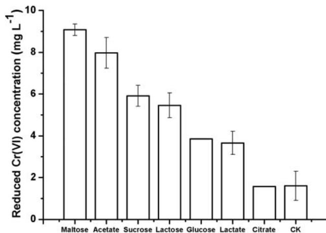
**Fig. 2.** Effects of carbon sources on the AQS-promoted Cr(VI) reduction. Strain Q5-1 reduced 10.4 mg L<sup>-1</sup> Cr(VI) in CDM medium with the addition of 155.1 mg L<sup>-1</sup> AQS and different carbon sources (maltose–citrate). CK represents Cr(VI) reduction in CDM medium amended with AQS. Error bars represent standard deviation of triplicate tests.
