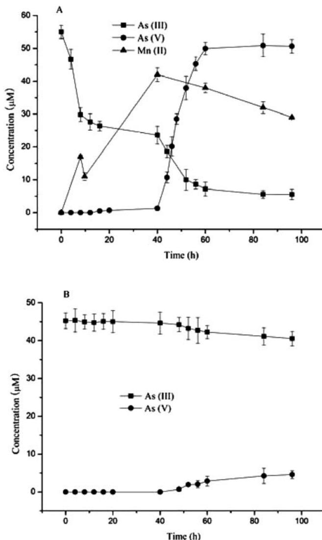
**Fig. 6.** Time course of As(III) oxidation using the biogenic Mn oxides generated by strain MnI7-9. A, 0.1 mmol biogenic Mn oxides added in 55  $\mu$ M NaAsO<sub>2</sub> solution; B, control experiments, 55  $\mu$ M NaAsO<sub>2</sub> solution without an addition of the biogenic Mn oxides; ■, As(III) concentration; ●, As(V) concentration; ▲, Mn(II) concentration.
