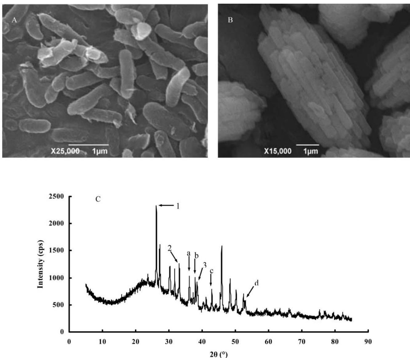
**Fig. 4.** A, SEM images of MnI7-9 cells cultivated in liquid A medium for 7 days without an addition of  $MnCl_2$ . B, SEM images of strain MnI7-9 incubated for 7 d and coated with the biogenic Mn oxides. C, XRD patterns of the biogenic Mn oxides generated by strain MnI7-9. Peaks a, b, c and d are typical of birnessite ( $\delta\text{-MnO}_2$ ); peaks 1, 2 and 3 are typical of manganite ( $\gamma\text{-MnOOH}$ ).
